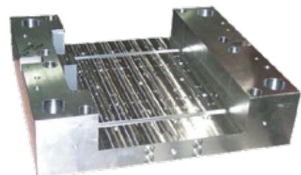
RoyAlloy plate shown after extensive pocket milling measured only 0.006" (0.15mm) distortion from corner to corner - plate size 6" x 28" x 32" (152mm x 711mm x 813mm).
